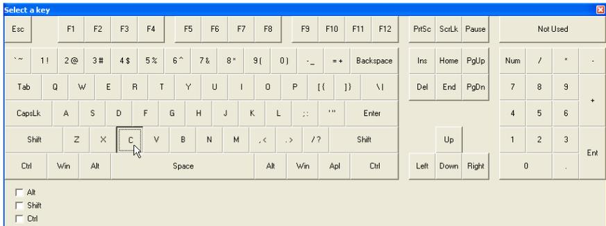
The KEAD6 has the capability to assign Shift, Ctrl, and Alt functions along with a keystroke. For example, one of the responses could be defined as the Ctrl+Alt+Del sequence. The keystrokes emulated by this combination have the same effect as holding the control and alt keys, then pressing the delete key on a PC keyboard. To create this input, check the Ctrl and Alt boxes on the lower left corner of the keyboard diagram, then click the Del button (shown below).
