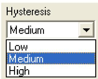
can be set to low. If, however, the potentiometer produces an unsteady reading, a setting of high should be used in order to keep unintentional keystrokes from being produced.
