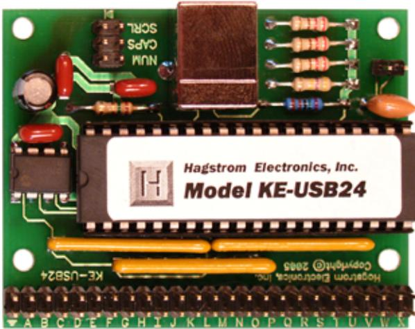
Use the KE-USB24 for interfacing keypads or switches to the PC's USB port to generate keystrokes.
