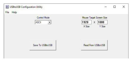
To configure the USBtoUSB, select the Control Mode from the dropdown box to choose the conversion mode. Select between ASCII (factory default), Extended ASCII, or Key Number Mode. See pages 3-9 for a description of each of the control modes.
