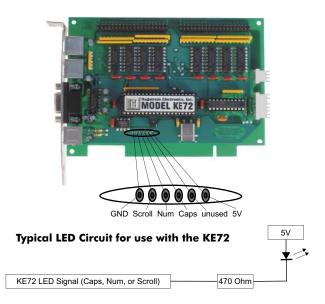
Keyboard status light drive is available with the KE72. The unit provides a connection point for the Num Lock, Caps Lock, and Scroll Lock status LEDs.
