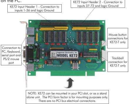
The KE72 uses standard drivers for its functions. No special software is required for the unit to work with your PC. Once programmed, the KE72 can be used with any PC compatible operating system.
