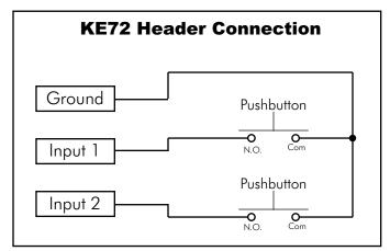
Electrical connection example for switches to KE72 inputs.
