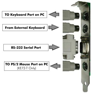
Note: Make connections to the KE72 with power off.
